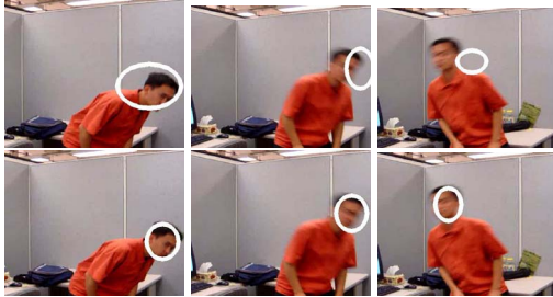
Fig. 3. Comparison of Condensation filter with our approach to fast motion. The first row is using Condensation filter. The second row is using our approach.
